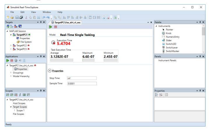
If you specify a sample time that is too small, a CPU overload can occur. If a CPU overload occurs, the target object property CPUOverload changes to detected. In that case, change **Fixed step size** to a larger value and rebuild the model.
